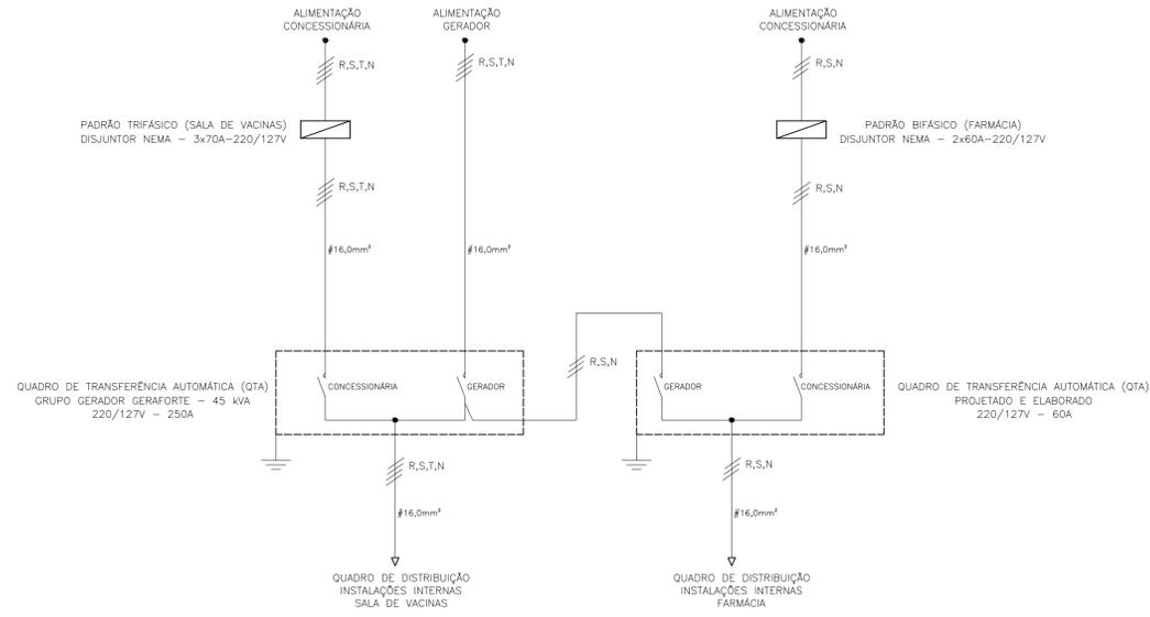
DIAGRAMA UNIFILAR SEM ESCALA
